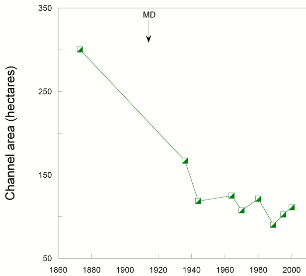
Figure 8. Active channel area change through time in (A) reaches of the Nooksack River, (B) White River (from Figure 6), and (C) Cedar River. “MD” in panel C marks the closing of Masonry Dam on the Cedar River, upstream of reach for shown in panel C. Data for panel A is from Collins and Sheikh (2004c); data for panel C is from Collins et al. (2003b).
